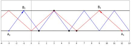
Examples of laser rays. Note that image contains two examples. The 3 sensors (denoted by black bold points on the tube sides) will register the blue ray but only 2 will register the red.
